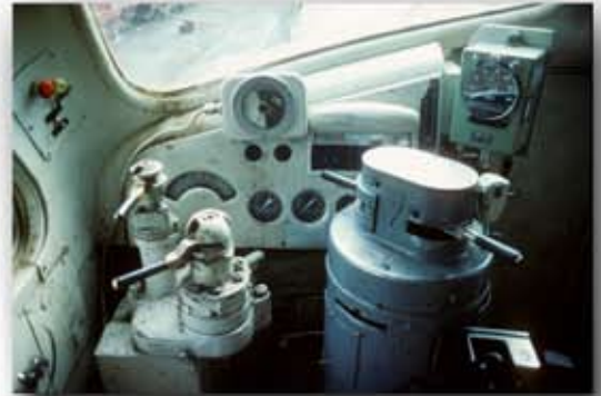
Above. The drivers side of a B class. Displayed is the A7EL brake valves (left) and what is known as a 'drum controller'. Below. Preserved B74 (Preserved by Seymour Railway Heritage Centre) at South Dynon, Melbourne.
